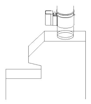
Fig. 7: Vent Damper Location
